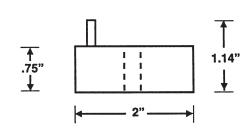
OPERATION: WHEN SWITCH CLOSES, LOAD ENERGIZES. WHEN SWITCH OPENS, LOAD DE-ENERGIZES AND THE TIME DELAY BEGINS, EVEN IF SWITCH RECLOSES DURING TIMING LOAD STAYS OFF UNTIL DELAY EXPIRES.
